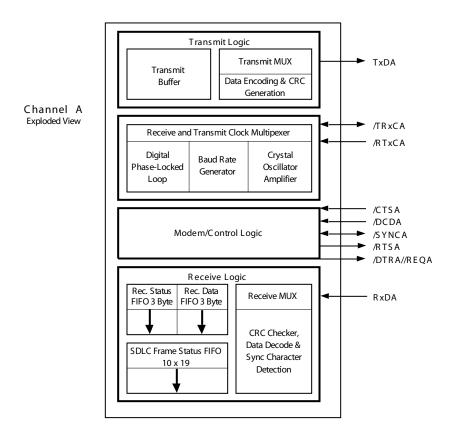
Figure 2. Channel A Exploded View
